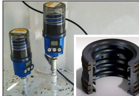
Chesterton Lubri-Cup™ EM and 615 HTG installed.
